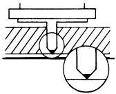
The welding cycle is activated by pressing the trigger switch on the gun. Current flowing through the fastener's high resistance point of contact creates instantaneous welds of extremely high strength.
