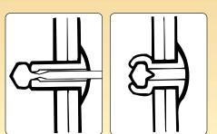
Back up washers for riveting in soft materials. Non-blind applications only. Install washer on rivet head protruding through backside of material to be fastened. Washers are zinc plated steel.
