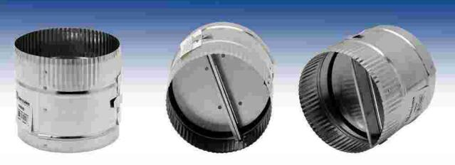
Backdraft dampers are used in ventilation systems to allow airflow in one direction and prevent airflow in the opposite direction. A pressure relief damper is developed with an elevated and adjustable start-open pressure while providing the backdraft function.
